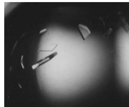
Figure 2 Photograph of RmlA crystals. These crystals have been grown in the presence of dTMP.
